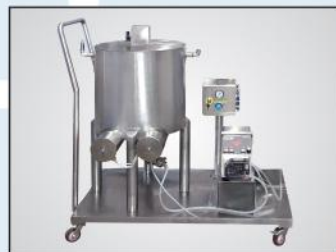
Peristaltic pump and solution holding tank
