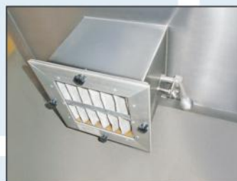
Inlet air filter & damper
