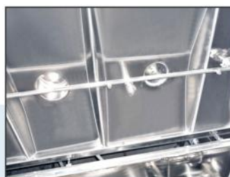
Top lid with spray nozzle & cip
