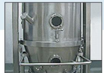
Product container & Expansion chamber assembly
